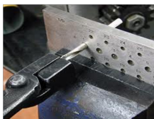
Draw plate for making wire.
